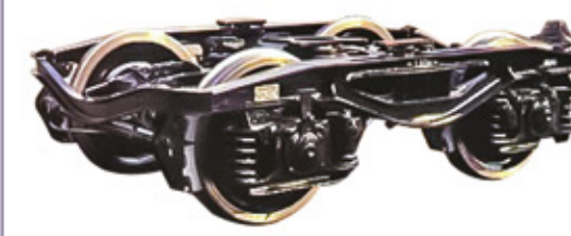
Y25 Bogie ▶ Gauge: 1435 mm | Axle Load: 22.5 T
