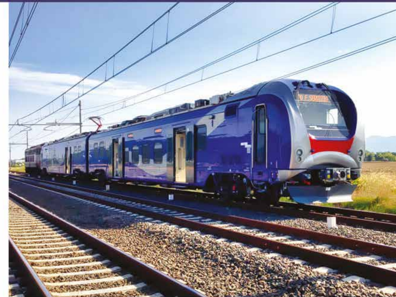
Single decker EMU Trainsets ▶ Gauge: 1435 | Design Speed: 160Km/h | Operating Speed: 140Km/h | Material - Aluminium
